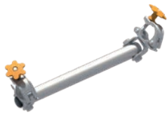
1248.261 Rotation lock, aluminium. Length 0.50 m, weight 2.8 kg.
