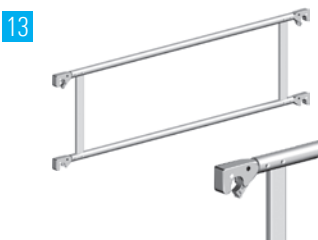
1206.180 Double guardrail 1.80 m aluminium. Length 1.80 m, height 0.50 m, weight 5.8 kg.
