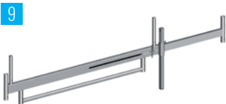
1338.320 Mobile beam with 2 spigots, 3.20 m, adjustable Steel rectangular tube, hot-dip-galvanized. For base widening in mobile working platforms. Width max. 3.20 m, min. 2.30 m, weight 42.6 kg.
